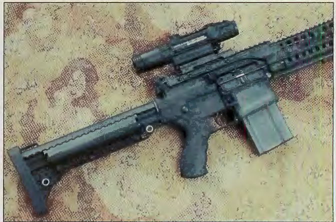
Here the Leupold CQ/T equipped AR-10 Carbine has the VLTOR A1 fixed stock, which also carries spare batteries. It proved far superior to the issue fixed stock.
